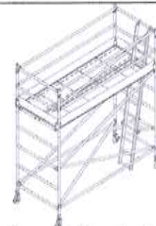
Figure 82 Plan Bracing
